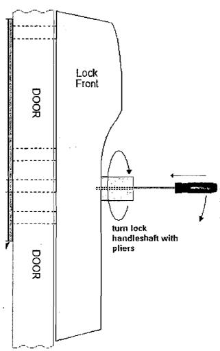
Push phillips head screwdriver into the drilled hole firmly AND then press downward on the screwdriver handle. While pushing in and pressing down on the screwdriver handle, turn the lock handle shaft with pliers.
